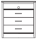
3418-137 Three Drawer Media Chest 36W x 22D x 38H in. 91W x 56D x 97H cm. Three Side-Guided Drawers, TV/VCR Shelf, Lumber Banded Laminate Top, Recessed Back, Wood Drawer Box.
