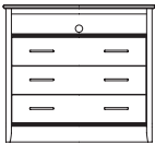
3418-139 Three Drawer Media Chest 42W x 22D x 38H in. 107W x 56D x 97H cm. Three Side-Guided Drawers, TV/VCR Shelf, Lumber Banded Laminate Top, Recessed Back, Wood Drawer Box.
